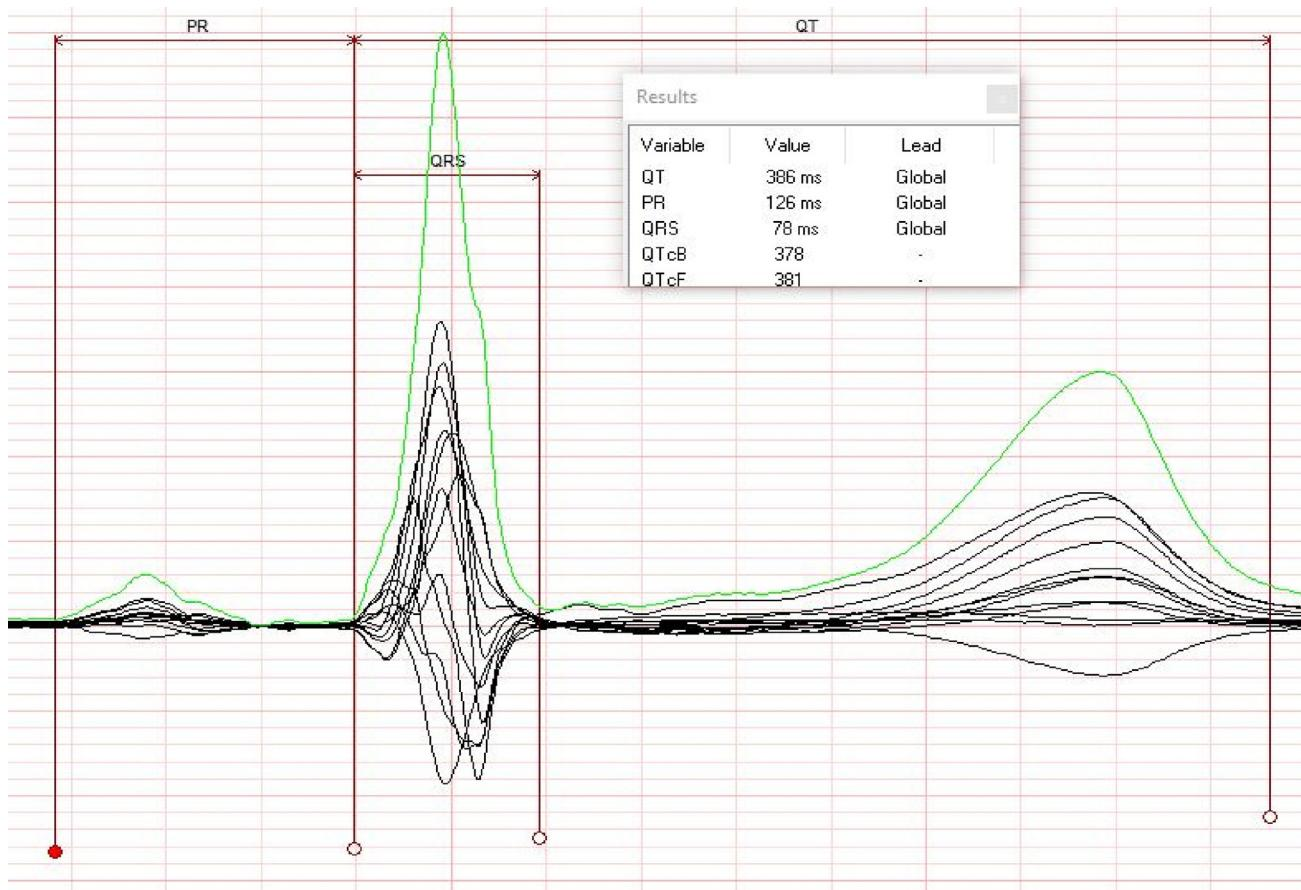
**Figure 3.** Superimposed median beat, with a display of vector magnitude (in green). Automatic calliper placements (PR, QRS and QT) and results (QT, PR, QRS, QTcB and QTcF), with the possibility of manual editing.
